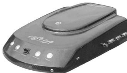
Figure 4.6. The G2010 "eagleeye" camera from Global Imaging Technologies also generates rectangular format frame images (Source: GIT).
