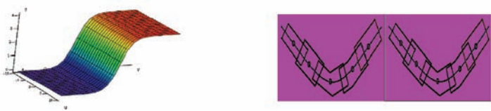
Figure 13.7. Left: Hyperbolic tangent function as model of an edge pair. Right: Overlapping break line patches (both from Brzank et al. (2005)). (N. Pfeifer et al., see page 181)
