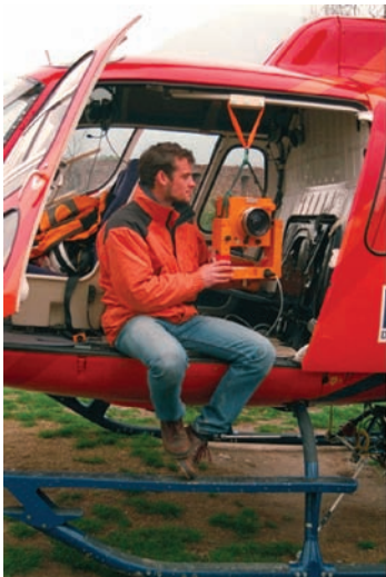
Figure 27.20. Zeiss UMK mounted in helicopter. (P. Patias et al., see page 376)
