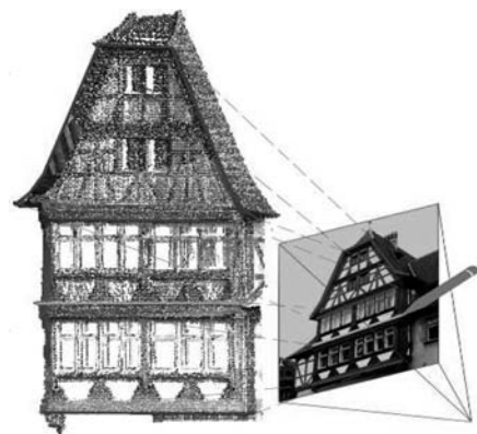
Figure 27.5. Monoplotted 3-D coordinates and lines onto the image in relation to the point cloud mesh. (see colour plate page 505)
