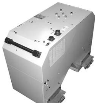
Figure 4.25. The ITRES Research CASI hyperspectral pushbroom line scanner (Source: ITRES Research).
