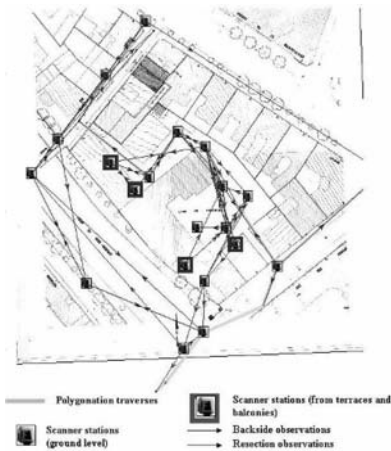
Figure 27.15(a). Ground control network used for the laser scanning survey. (see colour plate page 508)
