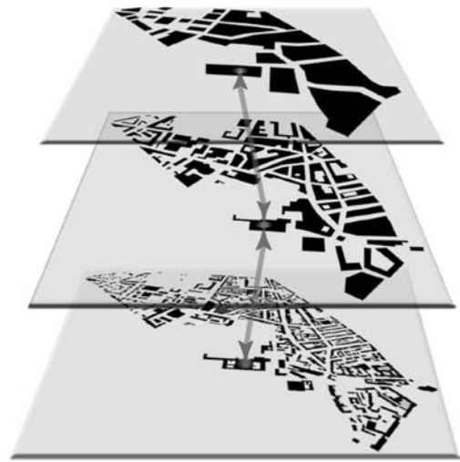
Figure 20.1. Example of an MRDB in three levels of detail; explicit links are shown for one object.
