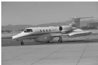
Figure 4.34. This Learjet aircraft is fitted with the STAR-3i interferometric SAR imager, which is housed in the prominent bulge on the underside of the aircraft (Source: Intermap).
