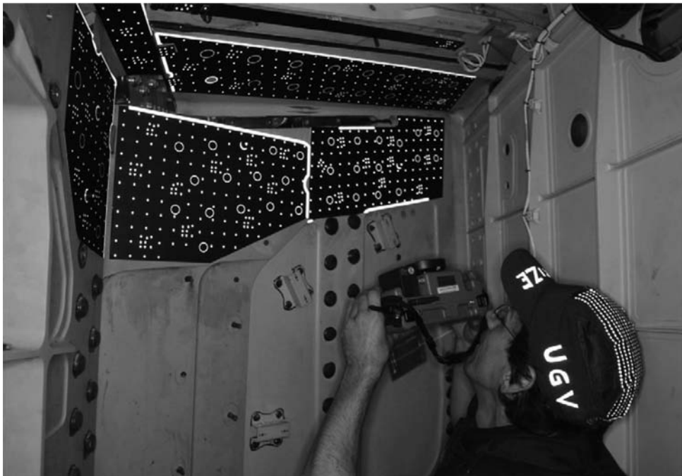
Figure 30.8. Photogrammetric measurement of the junction of the wing and fuselage in an Airbus A380 aircraft using a GSI V-STARS system. The photogrammetric system triggers an image processing function to automatically generate a 3-D surface and a 5 axis machining tool path. This process produces a titanium part that will fit in the corners. (Copyright: Airbus). (see colour plate page 513)
