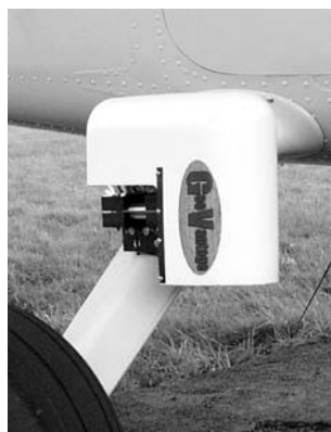
Figure 4.17. This GeoVantage multiple camera system comprising four small-format cameras has been fitted to the undercarriage of a light aircraft (Source: GeoVantage).
