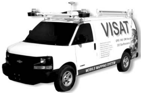
Figure 7.3. VISAT™ Van Mobile Mapping System. (see colour plate page 492)
