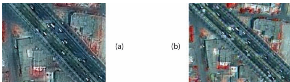
Figure 14.8. The wavelet fused Ikonos image using ERDAS Imagine 8.7 software. (a) Low-pass filtered fused data to remove artifacts; (b) Fused data without low-pass filtering. (Adopted from Boloorani et al., 2006) (Y. Zhang, see page 194)
