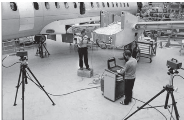
a) Example of a Metronor system being used to measure an aircraft engine mounting.
