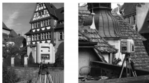
Figure 27.14(c). 3-D scanning system (Trimble GX). (see colour plate page 506)
