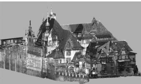
Figure 27.15(b). Final point cloud (with colours from the built-in video camera of the scanner). (see colour plate page 508)
