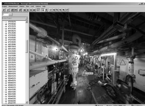
Figure 30.9. Left: Example sub-image from the panoramic “Hazmap” site measurement system showing further panoramic image locations as triangles. Right: Example integration with CAD where a new pipe design has been integrated into the Hazmap environment for clash detection. (Images Courtesy of Hazmap). (see colour plate page 514)
