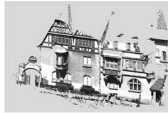
Figure 27.15(d). Point cloud (raw data) displayed with true colour pixels. (see colour plate page 508)
