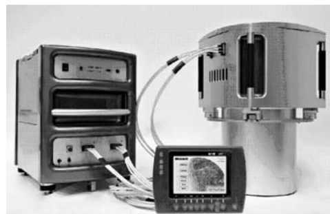
Figure 4.23. The current model of the Microsoft UltraCam-X camera is shown, comprising (from left to right) the control and data storage unit, the user's display screen and the camera unit (Source: Microsoft Photogrammetry).
