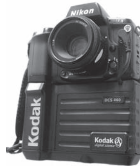
a) Kodak DCS 460 camera ( 3000 \times 2000 pixels).
