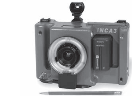
a) GIS INCA 3 photogrammetric metric camera.
