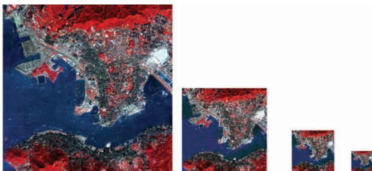
Figure 19.7. Scaling-up: Aggregation of digital images. (Z. Li, see page 272)
