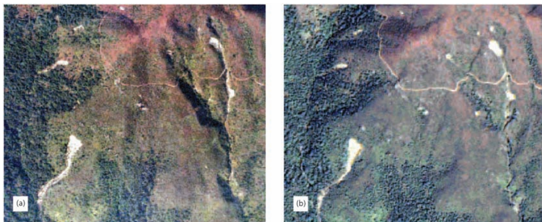
Figure 14.3. Comparison between aerial photograph and pan-sharpened Ikonos MS image showing landslide scars and patches of disturbed ground. (a) Aerial ortho-photograph (1:10 000); (b) Pan-sharpened Ikonos image (PCI Pansharp). (Adopted from Nichol and Wong 2005, subset) (Y. Zhang, see page 191)
