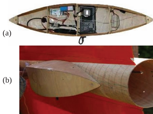
Figure 28.10. “Pod” with Ricoh GR digital camera (a), and “pod” position under the UAV (b). (P. Boccardo et al., see page 394)
