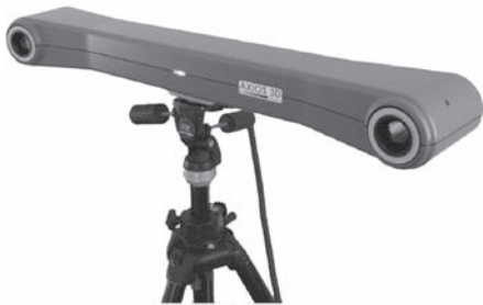
b) AXIOS 3-D CamBar stereo camera system.
