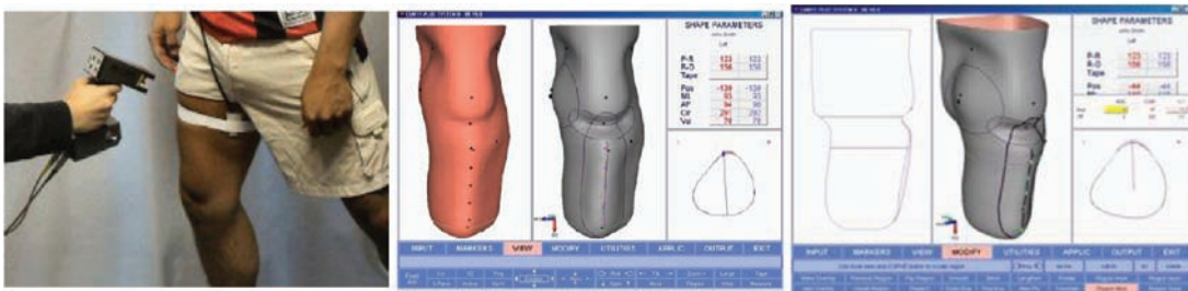
Figure 31.11. Lower limb socket design system CANFIT PLUS P&O: hand-held laser scanner and snapshots of the CAD/CAM solution. (N. D'Apuzzo et al., see page 432)
