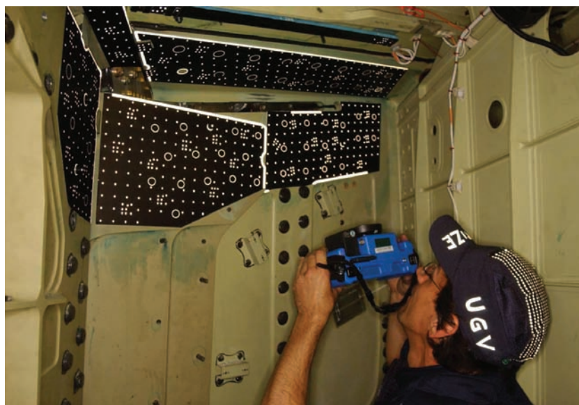
Figure 30.8. Photogrammetric measurement of the junction of the wing and fuselage in an Airbus A380 aircraft using a GSI V-STARS system. The photogrammetric system triggers an image processing function to automatically generate a 3-D surface and a 5 axis machining tool path. This process produces a titanium part that will fit in the corners. (Copyright: Airbus). (T. Luhmann et al., see page 418)
