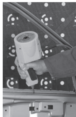
b) An AICON ProCam system being used to coordinate 3-D locations on a car door.
