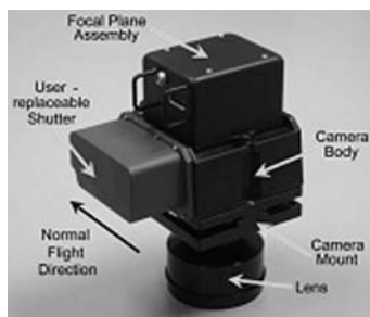
Figure 4.11. The new Leica RCD105 medium-format airborne digital frame camera (Source: Leica Geosystems).
