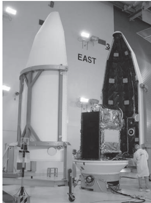
Figure 3.6. The Formosat-2 satellite is about to be enclosed within its protective heat shield prior to its launch at Vandenberg AFB, California (Source: NSPO, Taiwan).
