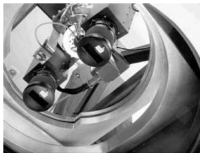
Figure 4.5. The New Metric Cameras that have been built for the GeoPIE project by the VTT research institute in Finland generate images with a rectangular format. This example comprises twin convergent cameras that are used to generate overlapping stereo frame images (Source: VTT).
