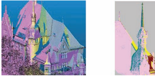
Figure 27.4. Different scans (colors) registered onto the same co-ordinate system. (P. Patias et al., see page 367)
