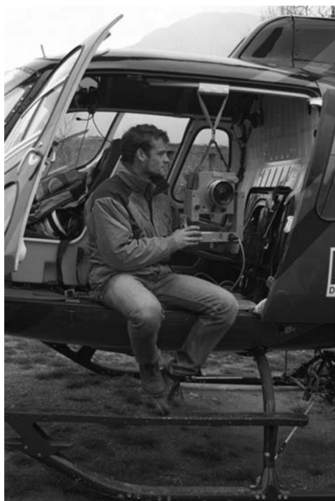
Figure 27.20. Zeiss UMK mounted in helicopter. (see colour plate page 509)
