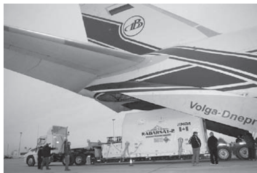
Figure 3.18. (Right) The Radarsat-2 satellite in its transportation box being loaded on to an Antonov An-224 freight aircraft for its flight to Baikonur, Kazakhstan where it was launched using a Russian Soyuz rocket in December 2007 (Source: Canadian Space Agency).
