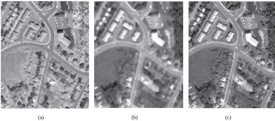
Figure 14.4. Fusion of QuickBird Pan and MS images for road extraction. (a) Original Pan image; (b) Original MS image; (c) Pan-sharpened MS image using UNB Pansharp (Adopted from Zhang et al. 2004, subsets). (see colour plate page 497)
