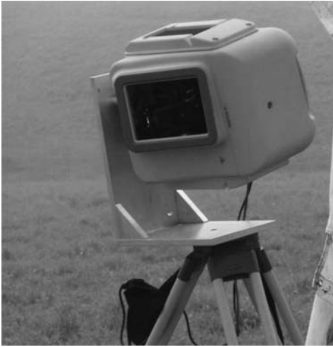
Figure 27.2. Trimble GX scanner with self-assembled adapter for excavations.
