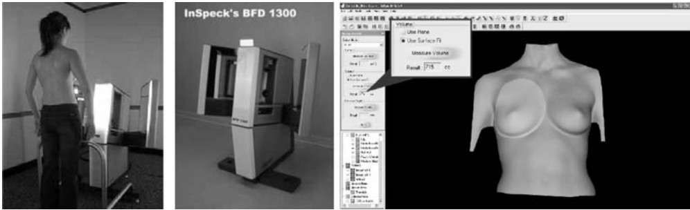
Figure 31.6. InSpeck Breast and Facial Digitizer BFD 1300 and measurement software EM-Measurement. (see colour plate page 516)
