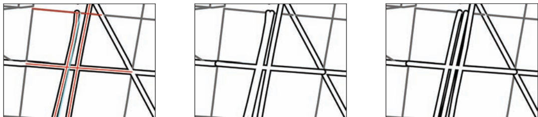
Figure 20.6. Insertion of new road (blue) (left); conflicts after applying signature (middle); situation after conflict resolution with displacement (right). (M. Sester, see page 285)
