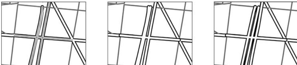
Figure 20.6. Insertion of new road (blue) (left); conflicts after applying signature (right); situation after conflict resolution with displacement (bottom). (see colour plate page 501)
