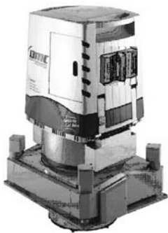
Figure 4.20. The latest version of the Intergraph DMC camera with its solid state disk (SSD) storage facility located on the side of the camera unit. The camera is mounted on a T-AS gyro-stabilized platform (Source: Intergraph).
